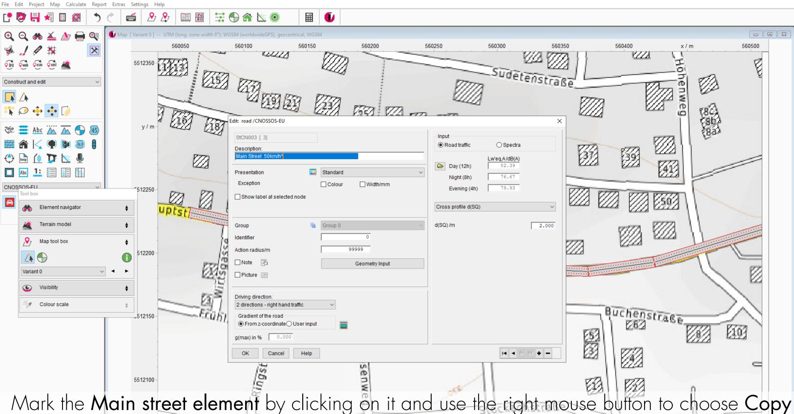
Mark the **Main street element** by clicking on it and use the right mouse button to choose **Copy element**. The input dialog box of the copied element will open. The name of copied element is marked with an \*.
