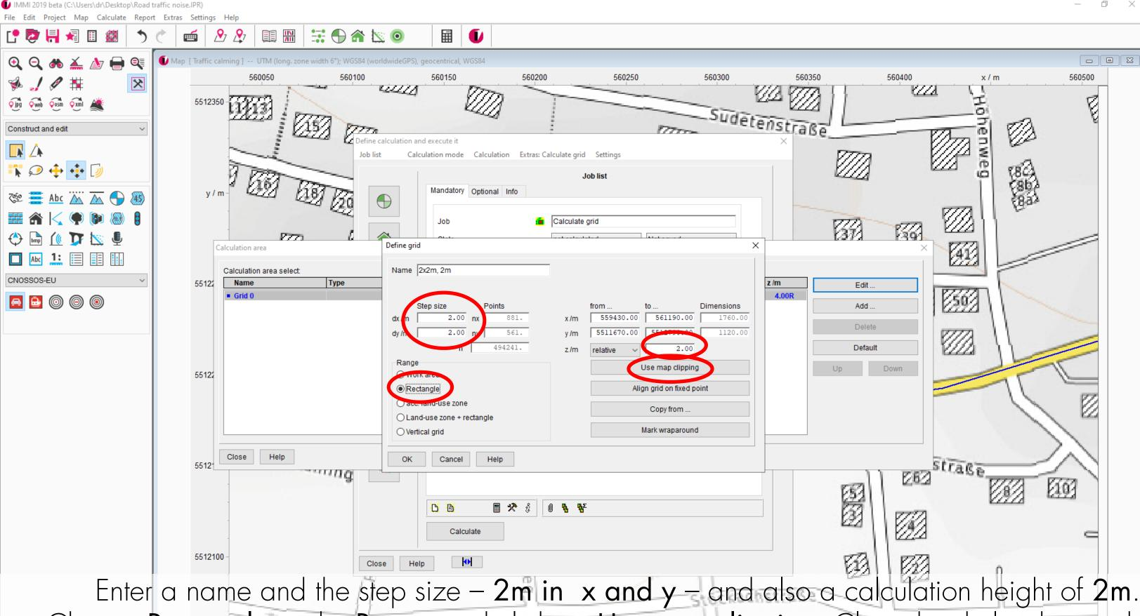
Enter a name and the step size -2m in x and y - and also a calculation height of 2m. Choose **Rectangle** as the **Range** and click on **Use map clipping**. Close the dialog box with 0k.
