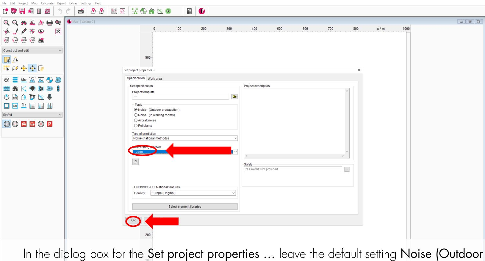
In the dialog box for the **Set project properties** ... leave the default setting **Noise** (Outdoor propagation) and choose **Lden** as the rating method. Close the dialog box by clicking on **OK**.
