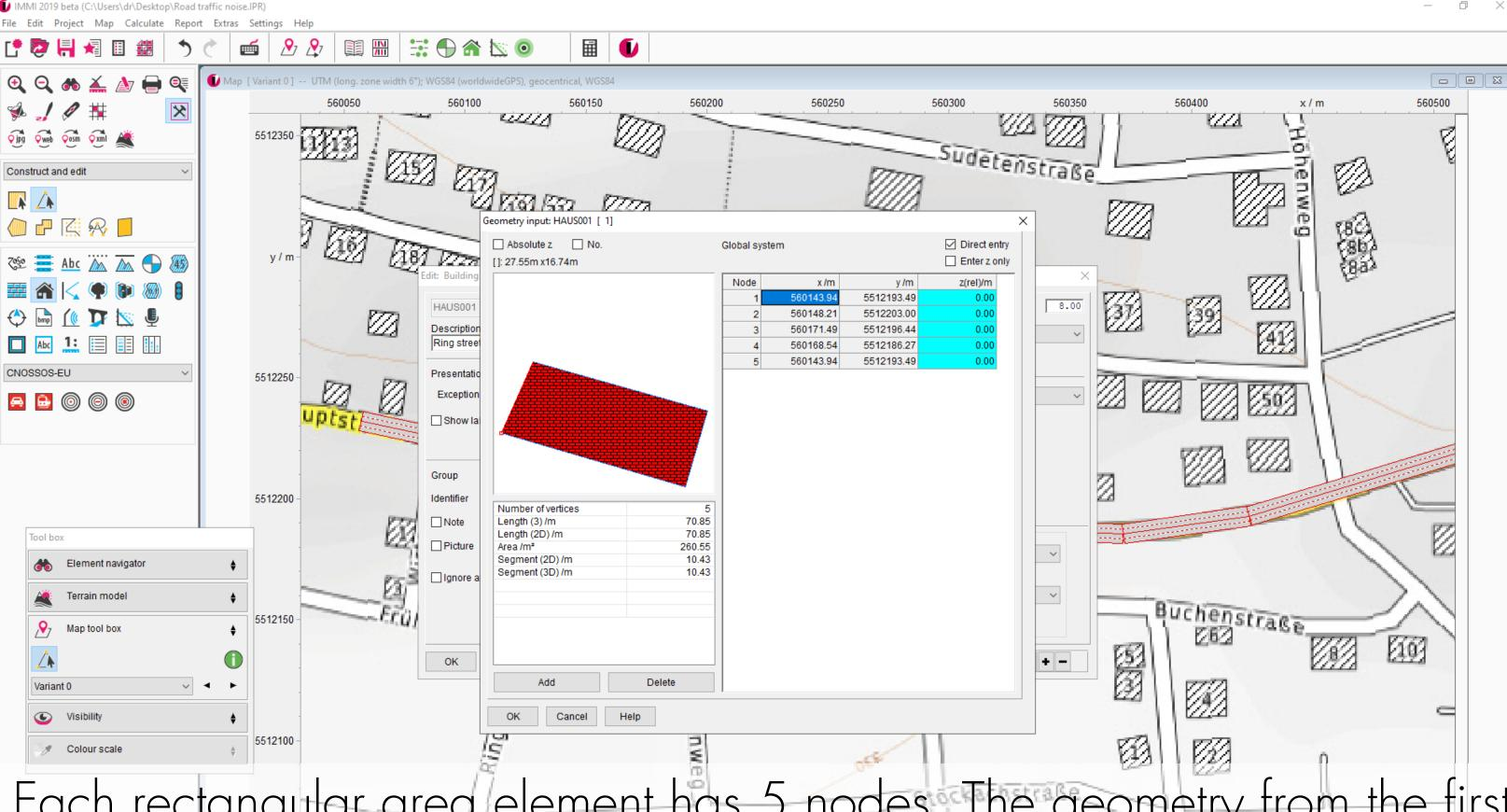
Each rectangular area element has 5 nodes. The geometry from the first and the fifth node is the same. Close the dialog box with **OK**.
