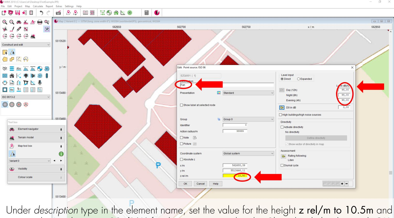
Under description type in the element name, set the value for the height z rel/m to 10.5m and set the Level input to 98 dB(A) for day, evening and night. Close the dialog box with OK.
