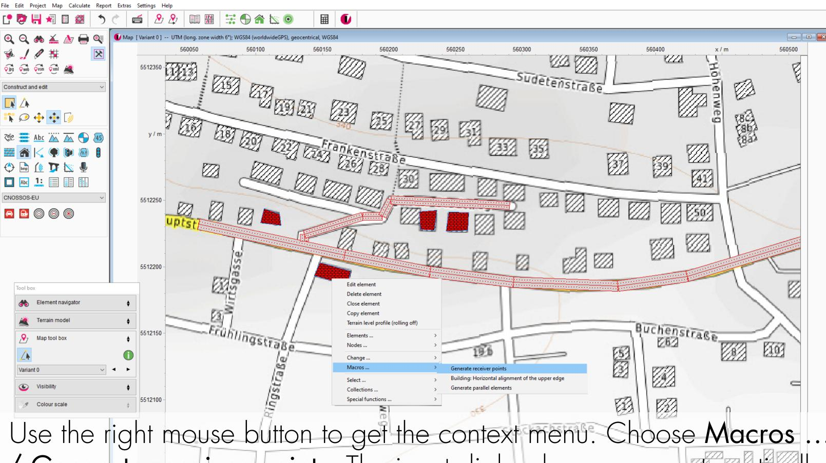
/ Generate receiver points. The input dialog box opens automatical
